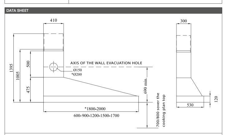
Please do not connect the hood to an air extraction pipe smaller than the advised one. Danger of a general bad working of the appliance and overheating of the engine. In the case the extraction pipe cannot be  $\emptyset$  200mm (1200mc/h) and the hood is larger than 180 cm, we suggest to order the hood with an engine apt to air extraction pipe  $\emptyset$  150mm (900mc/h)
